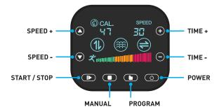
Your 4D vibration plate can be controlled with either the touch screen panel or the wearable remote control. There are 7 manual settings and 3 programmed settings [P1, P2, P3].
